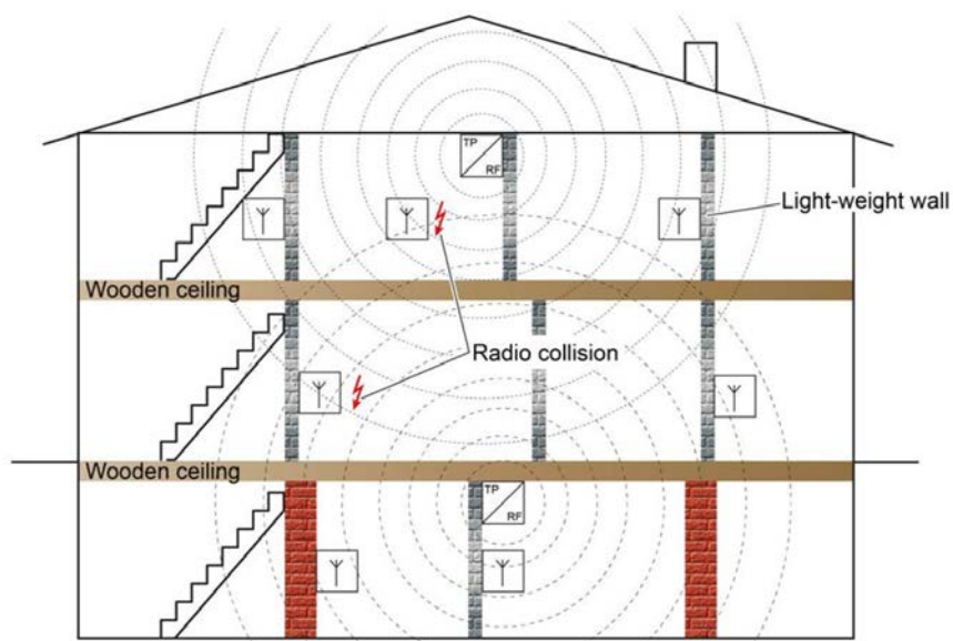
Figure 20: Building structure with two KNX RF lines, unfavourable interference
